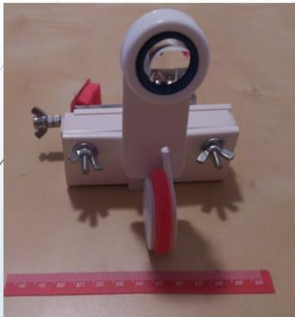
First device: Lente de Volk with smartphone to examine foreground of the eye
